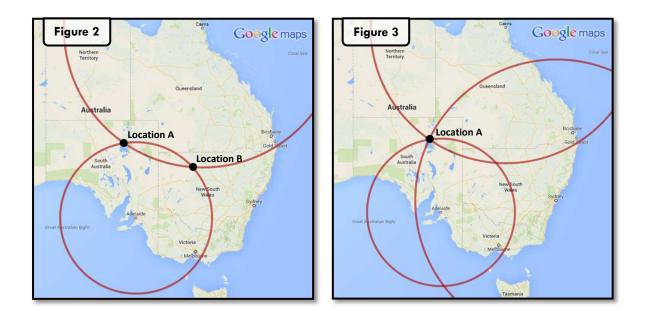
Trilateration also works in three-dimensions as well, but involves using spheres instead of circles and requires *four* distances to form a unique solution instead of three. GPS receivers use three-dimensional trilateration to tell you A) where you are on the earth and B) your current height.
